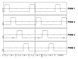
FIGURE 2. FOUR PHASE PWM OUTPUT AT 500kHz
