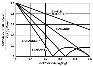
FIGURE 14. RIPPLE CURRENT vs DUTY CYCLE
