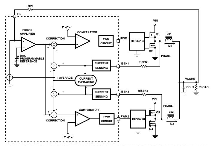
FIGURE 1. SIMPLIFIED BLOCK DIAGRAM OF THE HIP6301V VOLTAGE AND CURRENT CONTROL LOOPS FOR 2-PHASE REGULATOR
