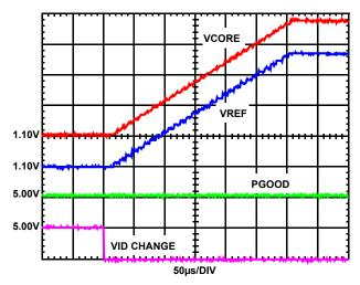
FIGURE 7. VCORE TRACKING THE REFERENCE VOLTAGE
