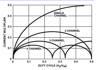
FIGURE 15. CURRENT MULTIPLIER vs DUTY CYCLE
