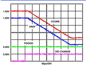
FIGURE 6. VCORE TRACKING THE REFERENCE VOLTAGE
