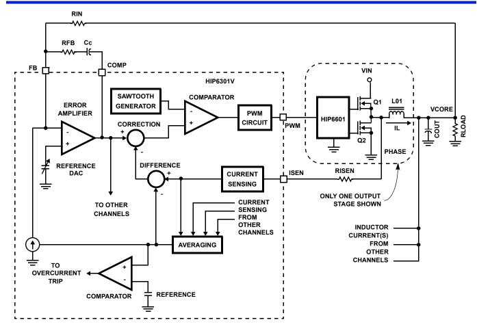
FIGURE 9. SIMPLIFIED FUNCTIONAL BLOCK DIAGRAM SHOWING CURRENT AND VOLTAGE SAMPLING
