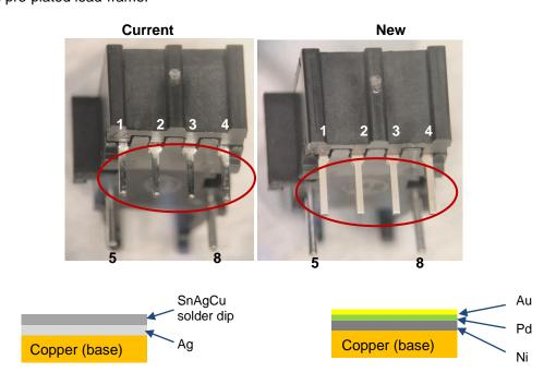
Active pins (pin1 to pin4 in red circle): Affected by changing to new NiPdAu lead-frame finish.
