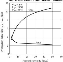
Fig.10-b Propagation Delay Time vs. Forward Current
