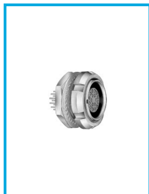
ECG.2G Fixed socket with two nuts, key (G), straight contact for printed circuit (back panel mounting)
