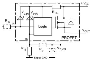
$R_{bb}$  = 120  $\Omega$  typ.,  $V_{Z,IN}$  =  $V_{Z,IS}$  = 74 V typ.,  $R_{IS}$  = 1 k $\Omega$  nominal. Note that when over voltage exceeds 79 V typ. a voltage above 5V can occur between IS and GND, if  $R_V$ ,  $V_{Z,VIS}$  are not used.
