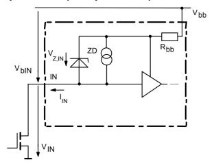
When the device is switched off ( $I_{IN} = 0$ ) the voltage between IN and GND reaches almost  $V_{bb}$ . Use a bipolar or MOS transistor with appropriate breakdown voltage as driver.
