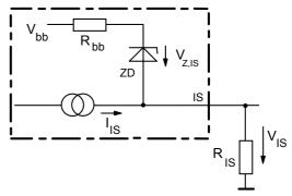
$V_{\rm Z,IS}$  = 74 V (typ.),  $R_{\rm IS}$  = 1 k $\Omega$  nominal (or 1 k $\Omega$  /n, if n devices are connected in parallel).  $I_{\rm S}$  =  $I_{\rm L}/I_{\rm liis}$  can be driven only by the internal circuit as long as  $V_{\rm out}$  -  $V_{\rm IS}$  > 5 V. If you want measure load currents up to  $I_{\rm L(M)}$ ,  $R_{\rm IS}$
