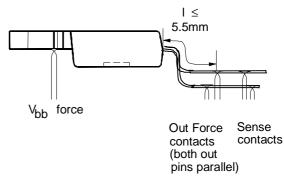
Typical RON for SMD version is about 0.2 m $\Omega$  less than straight leads due to I  $\approx$  2 mm
