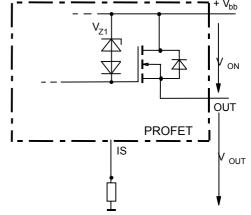
$V_{ON}$  is clamped to  $V_{ON(Cl)} = 62 \text{ V}$  typ
