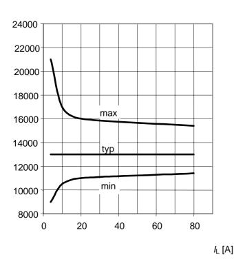
Current sense ratio:  $K_{\text{ILIS}} = f(I_{\text{L}}), T_{\text{j}} = 150^{\circ}\text{C}$
