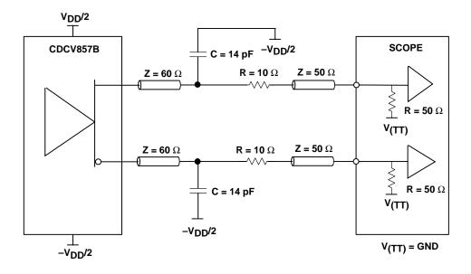
Figure 2. Output Load Test Circuit
