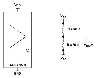
Figure 1. IBIS Model Output Load
