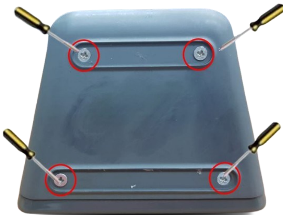
Figure 19 - Remove Screws To Detach Bottom Cover
