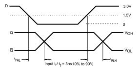
FIGURE 1. LVTTL to Differential LVPECL Propagation Delay
