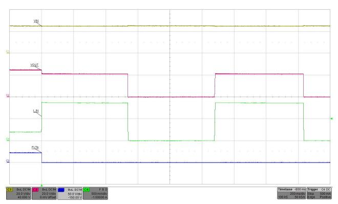
Figure 3. J4 = 1-2 Position, Current Limit (800 mA) and Auto-Retry
