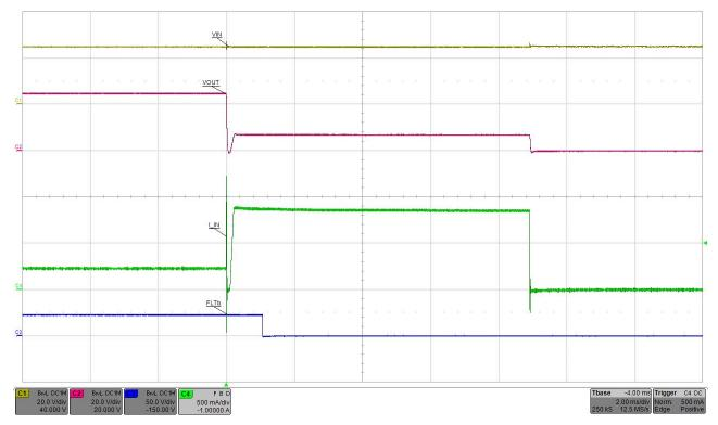
Figure 4. Output Short-Circuit Protection
