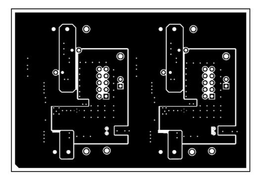
Figure 8. TPS26624-25EVM Bottom Layer Routing
