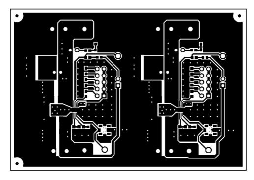
Figure 7. TPS26624-25EVM Top Layer Routing
