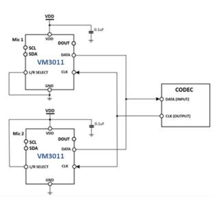
Typical Application Circuit for Stereo Microphone Configuration
