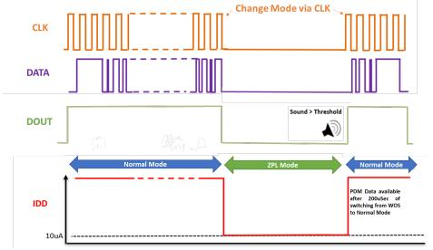
Switching between different microphone modes using PDM CLK
