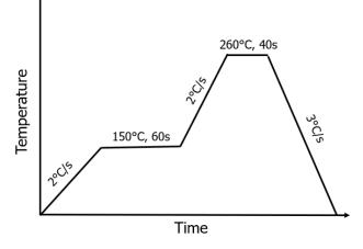
Figure 6: Solder Reflow Profile
