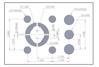
Solder Stencil Pattern – All dimensions are in mm
