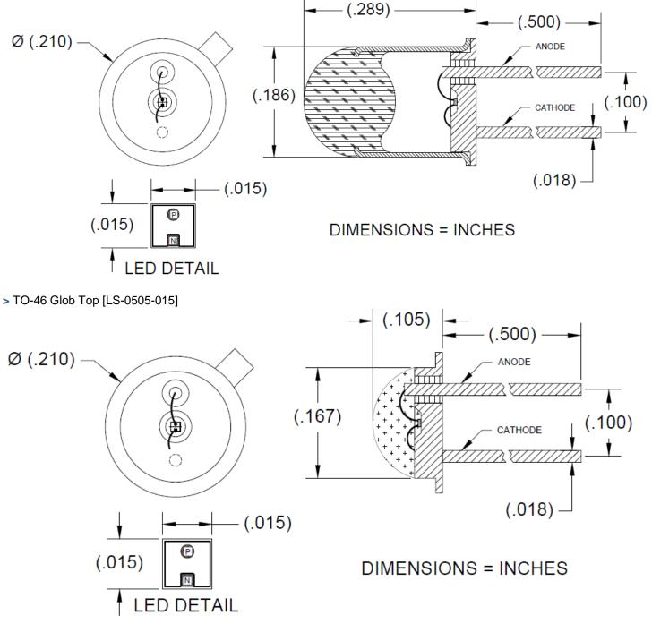
>Soldering Conditions: 260°C 1/16 inch away from case for 3 seconds max.
