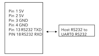
Note: If RS232 is not required, the MK-043R can be hardware configured to utilize UART0 as another TTL-level UART in addition to UART1. Please contact our support department at support@amuletechnologies.com for details. For I/O requirements through SPI or  $I^2C$ , also contact Amulet's support department.
