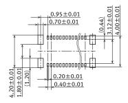
Recommended metal mask pattern Metal mask thickness: When 120 µm (Terminal opening ratio: 60%) (Metal-part opening ratio: 100%)
