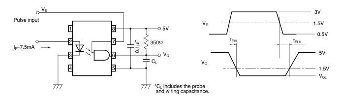
Fig.3 Test Circuit for Instantaneous Common Mode Rejection Voltage
