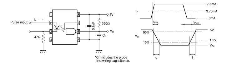
Fig.2 Test Circuit for Enable Propagation Delay Time
