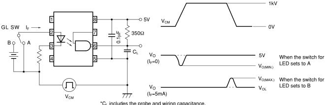
\*C<sub>L</sub> includes the probe and wiring capacitance.
