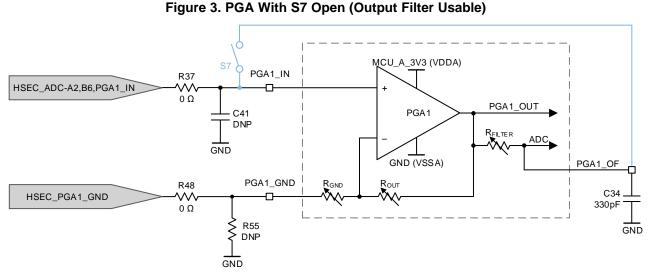
The S7 switch bank provides the flexibility to either use the PGA output filter pin (PGAn\_OF) for filtering (S7 open in Figure 3) or for sampling the PGA input voltage directly by bypassing the internal PGA (S7 closed in Figure 4).
