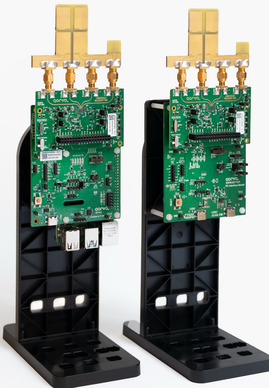
Raspberry Pi 4 and QM35825 Radio Board
