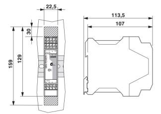
Mounting position: Installation depth 107 mm (+ DIN rail)
