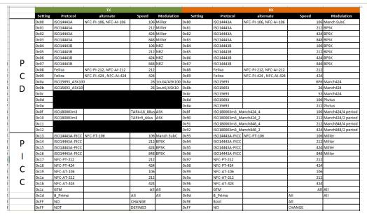
Figure 20. RF Protocol configuration indexes
