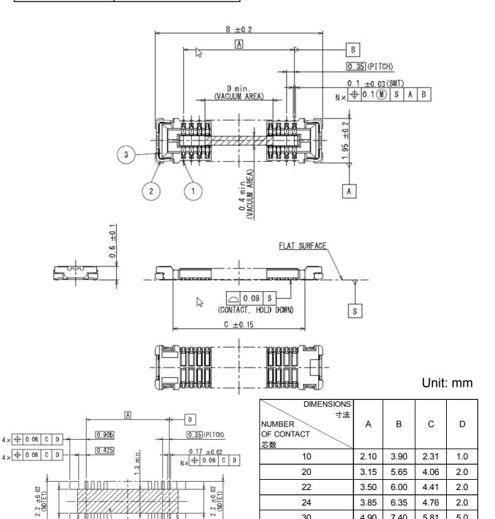
Note 1) Dimension 2.8  $\pm$  0.02 is recommended in case repair is needed.
