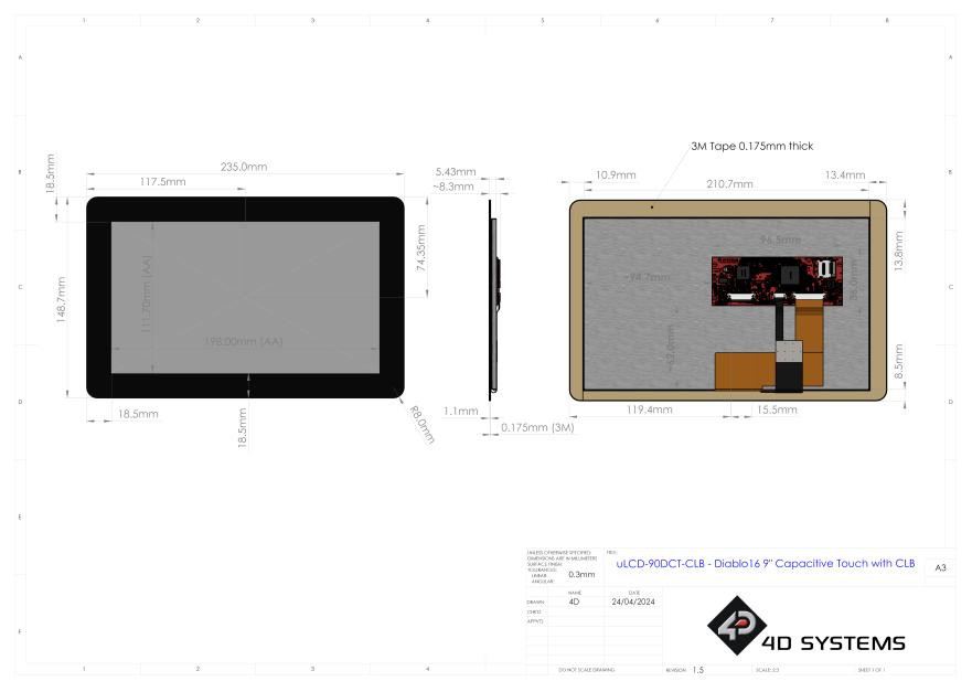
uLCD-90D Series Schematic Details (HW REV 1.5)
