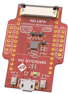
The 4D-UPA is a single module with a micro USB interface, and DIP-style pads for GPIO breakout of all the signals used on the Display interface, which is useful for development or final product use. Standard 2.54mm (0.1") male pin headers can be mounted so the module signals can be interfaced easily.
