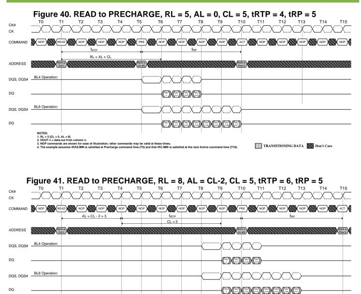
NOTES: 1. RL = 8 (CL = 5, AL = CL - 2) 2. DOUT n = data-out from column n. 3. NOP commands are shown for ease of illustration; other commands may be valid at these times. 4. The example assumes tRAS.MIN is satisfied at Precharge command time (T10) and that tRC.MIN is satisfied at the next Active command time (T15).
