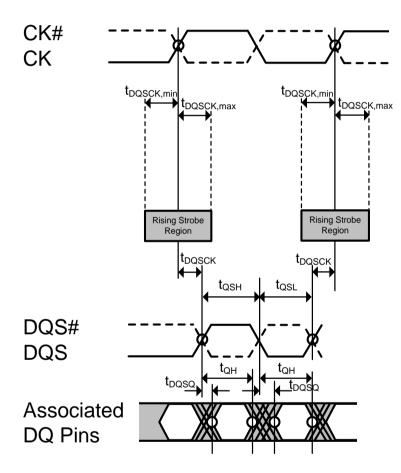
Figure 18. READ timing Definition
