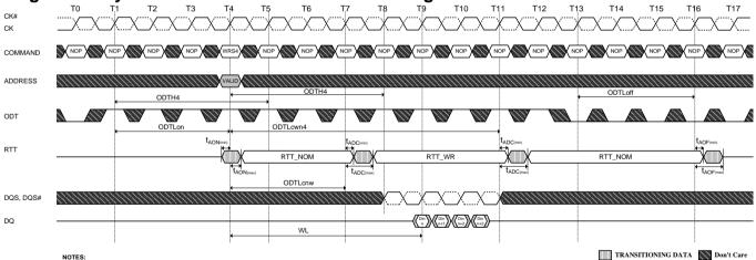
NOTES: Example for BC4 (via MRS or OTF); AL = 0, CWL = 5. ODTH4 applies to first registering ODT high and to the registration of the Write comm In this example, ODTH4 would be satisfied if ODT went low at T6 (4 clocks after the Write command).
