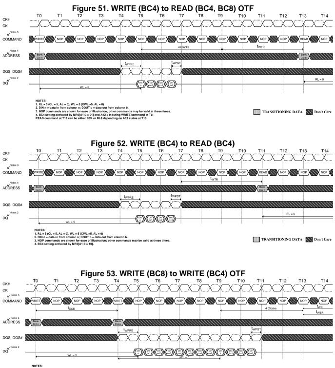
NOTES: 1. WL = 5 (CWL = 5, AL = 0) 2. DIN n (or b) = data-in from column n (or column b). 3. NOP commands are shown for ease of illustration; other commands may be valid at these times. 4. BL8 setting activated by MR0[A1:0 = 01] and A12 = 1 during WRITE command at T0. BC4 setting activated by MR0[A1:0 = 01] and A12 = 0 during WRITE command at T4.
