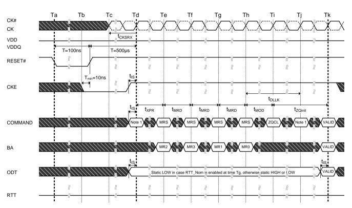
Figure 5. Reset Procedure at Power Stable Condition
