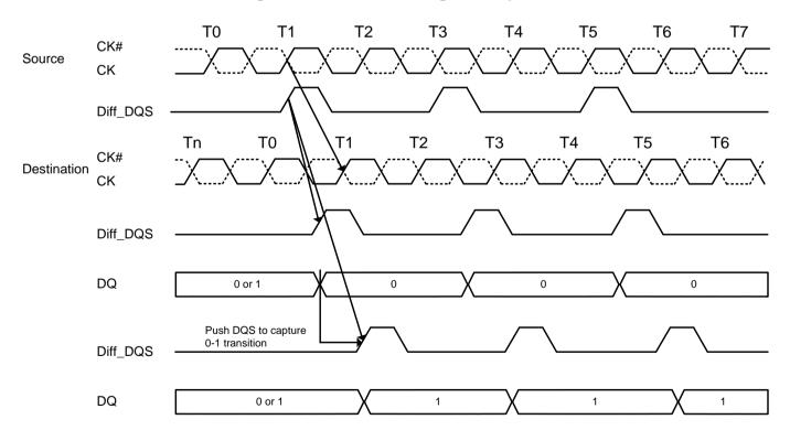
Figure 13. Write Leveling Concept
