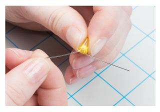
Once all bending is complete, place the LED on a table or flat surface to make sure it sits flat and upright. If not, make any adjustments now.
