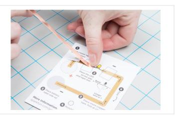
This template includes a few turns - to keep a solid connection of copper around corners, we'll be using a folding technique to press the tape into shape. Start by sticking the copper tape down until you reach the corner, then fold the tape backward on itself. Use a fingernail or pen to give it a good crease at the edge.
