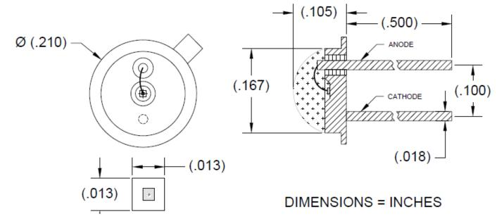
>Soldering Conditions: 260°C 1/16 inch away from case for 3 seconds max.
