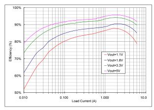
Condition:  $V_{IN} = 12 \text{ V}$   $C_{OUT} = 88 \text{ } \mu\text{F} \text{ } (22 \text{ } \mu\text{F} \text{ x 4})$  Frequency = 600 kHz  $L_{OUT} = 1.0 \text{ } \mu\text{H} \text{ } (V_{OUT} = 1.1 \text{ V & 1.8 V})$   $L_{OUT} = 2.2 \text{ } \mu\text{H} \text{ } (V_{OUT} = 3.3 \text{ V})$   $L_{OUT} = 3.3 \text{ } \mu\text{H} \text{ } (V_{OUT} = 5 \text{ V})$
