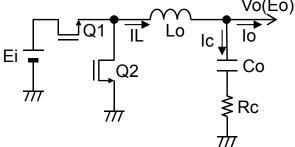
Figure 7-1: Output ripple for output inductor and capacitor
