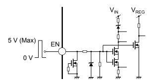
Figure 5-1: Internal circuit with EN pin
