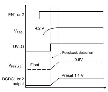
Figure 2-2: Internal feedback operation
