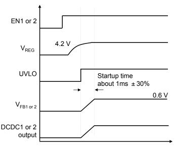
Figure 2-3: Soft Start (SS) Operation
