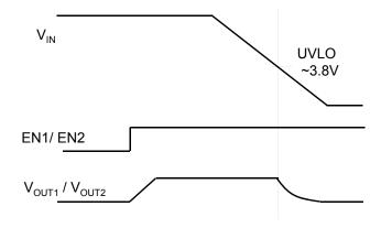
Figure 6-2 : V<sub>IN</sub> power down sequence
