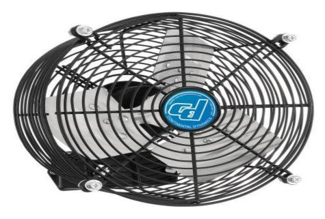
The guard mount exhaust fan is designed for low-pressure exhausting and cooling applications. Steel spiral wire guards enclose 3 aluminum fan blades for safety. Wire guards feature built-in mounting holes for easy installation. The 120V, single phase totally enclosed motor is permanently lubricated for long life. It is UL, cUL listed and conforms to UL507 standard.
