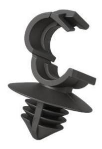
Hinged locking clamp securely holds corrugated or convoluted tubing and other bundles. It has an internal rib spanning the diameter of the clamp providing a tight grip and has a releasable latch that is convenient for maintenance or re-routing. The large base ensure stable mounting.
