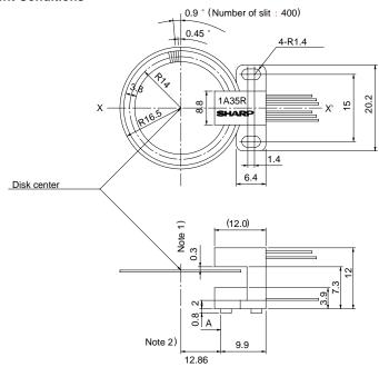
Note 1) Distance between disk surface and case surface in the detector side is 0.3mm.
