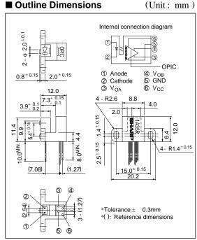
\*" OPIC" (Optical IC ) is a trademark of the SHARP Corporation. An OPIC consists of a light-detecting element and signalprocessing circuit integrated onto a single chip.
