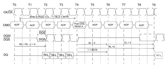
The minimum number of clocks from the burst write command to the burst read command is [CL - 1 +BL/2 + t<sub>WTR</sub>]
