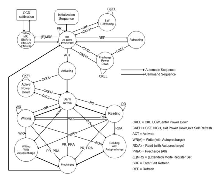
Note: Use caution with this diagram. It is intended to provide a floorplan of the possible state transitions and the commands to control them, not all details. In particular situations involving more than one bank, enabling/disabling on-die termination, Power Down entry/exit – among other things – are not captured in full detail.
