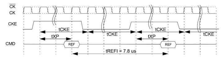
The pattern shown above can repeat over a long period of time. With this pattern, DRAM guarantees all AC and DC timing & voltage specifications and DLL operation with temperature and voltage drift.
