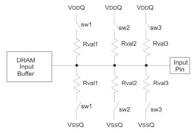
Switch (sw1, sw2, sw3) is enabled by ODT pin.
