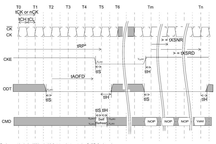
Device must be in the "All banks idle" state prior to entering Self Refresh mode.
