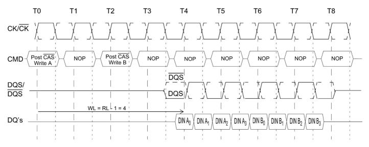
The seamless burst write operation is supported by enabling a write command every other clock for BL = 4 operation, every four clocks for BL = 8 operation. This operation is allowed regardless of same or different banks as long as the banks are activated.
