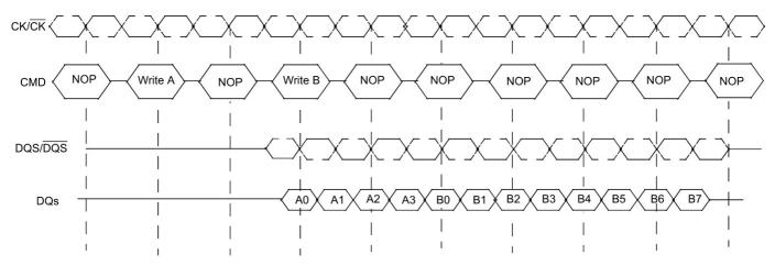
Write burst interrupt function is only allowed on burst of 8. Burst interrupt of 4 is prohibited.
