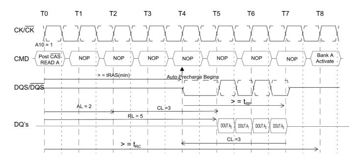
Burst read with auto precharge followed by an activation to the same bank ( $t_{RP}$  Limit): RL = 5 (AL = 2, CL = 3, internal  $t_{RCD} = 3$ , BL = 4,  $t_{RTP} <= 2$  clocks)
