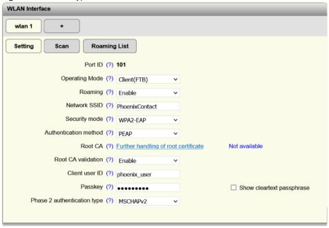
Table 4-3 Encryption: WPA2-EAP and FT-EAP: Parameters
