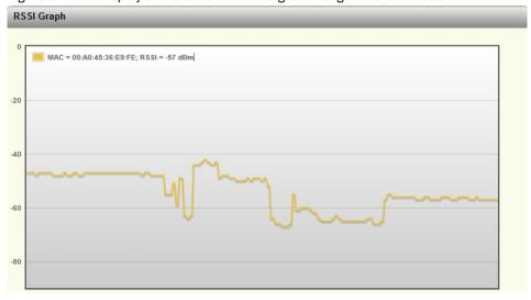
Figure 3-26 Display of the current WLAN signal strength in Client mode
