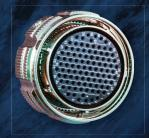
EMI shielding: Glenair incorporates ground springs in receptacle connectors and grounding fingers in special coupling nut-equipped plugs to optimize 360° shell-to-shell continuity.
