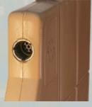
The STAR-PAN system uses Glenair Mighty Mouse 807 connectors which are fully-compliant to US and NATO standards for EUDs, radios, batteries, and C4ISR peripherals. Many soldier batteries can be directly connected to the STAR-PAN system without adapters using the general-purpose Mighty-Mouse equipped C1 cable.
