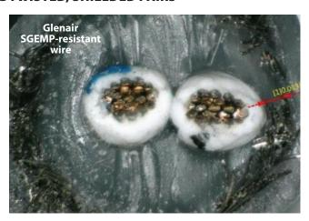
M27500 wire (left) cross-section shows numerous air gaps. Glenair SGEMP resistant wire (right), with Duralectric EMP low-Z filling material has no air gaps. ArmorLite braided shielding with minimum 95% coverage protects against secondary gamma radiation and electrons
