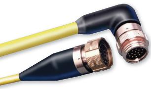
Geo-Marine® plugs are equipped with arctic coupling nuts—made from marine-grade naval bronze—with easy-to-grip castellated knurling and a powerful ratcheted anti-decoupling mechanism which guarantees reliable mating and demating performance in even the harshest environments. Supplied as discrete connectors—or more typically in build-to-print overmolded cable assemblies.
