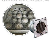
Connectors utilizing CODE RED hermetic encapsulant sealing underwent a grueling qualification test and validation process to prove material durability and hermeticity. Validation testing including 100 cycles of thermal shock IAW EIA-364-32 Test Condition A -65°C to +200°C while maintaining hermeticity followed by 1000 hours of thermal aging at 200°C. Additional tests included:
