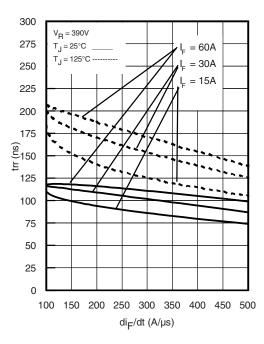
Fig. 5 - Typical Reverse Recovery Time vs. dl<sub>F</sub>/dt (Per Leg)
