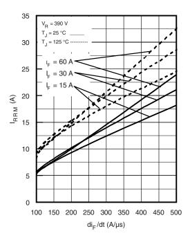
Fig. 6 - Typical Recovery Current vs. dI<sub>F</sub>/dt (Per Leg)
