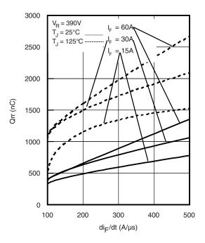
Fig. 7 - Typical Stored Charge vs. dl<sub>F</sub>/dt (Per Leg)
