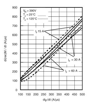
Fig. 8 - Typical  $dI_{(rec)M}/dt$  vs.  $dI_F/dt$  (Per Leg)
