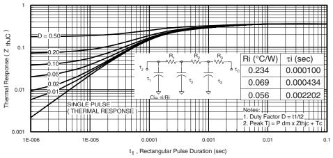
Fig. 4 - Maximum Thermal Impedance  $Z_{\text{thJC}}$  Characteristics
