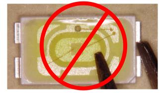
(2) In general, LEDs should only be handled from the side. This also applies to LEDs without a silicone sealant, since the surface can also become scratched.
