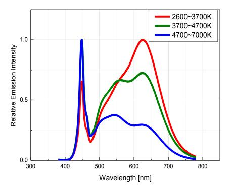
Fig 2. Radiant Pattern, T<sub>j</sub>= 25°C, I<sub>F</sub>=65mA
