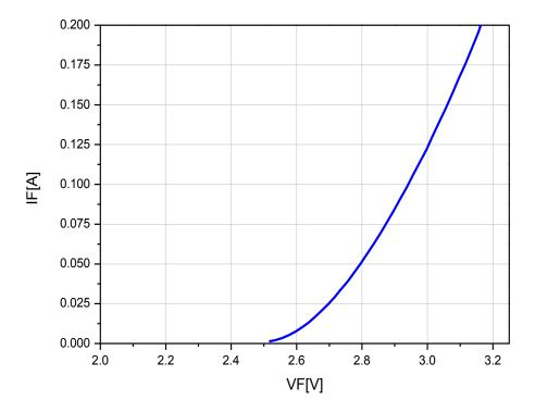
Fig 3. Forward Voltage vs. Forward Current, T<sub>j</sub>= 25°C
