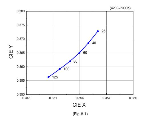
Fig 8. Chromaticity Coordinate vs. Junction Temperature,  $I_F$ =65mA
