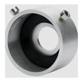
The Tallysman Screw Compression Pipe Mount Adapter is designed to fit all of our TW3000 family of antennas. It is meant for use with the customer's existing non-standard pipe (maximum pipe size of 40 - 42 mm (1.5 inch inside diameter)) and is secured with 2 stainless steel cap screws. Our antenna is secured to the adapter with 2 hexagonal nuts.
