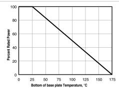
Derating (thermal resistance): 0.666W/°K (1.5KWV). Without a heatsink, when in free air at 25°C, the TEH100 is rated for 3.5W. Derating for temp. above 25°C is 0.0234W/°K.
