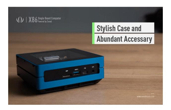
With **Dual Gigabit Ethernet**, you can build the OpenWrt project and pfSense with ease. There are **also two of M.2 PCle (B Key and M Key)**, which enables various expandable capabilities including Hard Drives, SSD, GPU, 4G, and even 5G cellular network connectivity.
