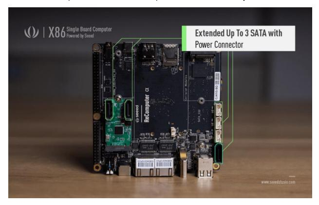
With ODYSSEY - X86J4125, you can build your own NAS (Network-Attached Storage), your high-performance Virtual Router, or a 4G LTE Gateway in your IoT applications. There is an onboard ATSAMD21 Core, an ARM Cortex-M0+ MCU that allows you to program Arduino on the x86 platform. The Raspberry Pi compatible 40-Pin provides hardware compatibility to most of the Pi HATs in the market. All of these features providing endless possibilities of using the ODYSSEY - X86J4125.
