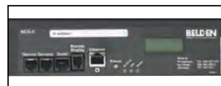
Intelligent PDU Communication and Environmental Monitoring Ports
