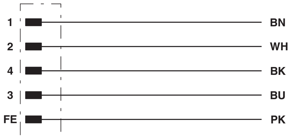
Contact assignment of the M12 plug
