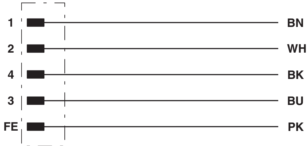
Contact assignment of the M12 plug
