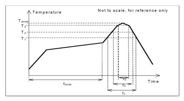
Fig 1.0, this profile is the minimum requirement for evaluating soldering heat resistance of components. Heat transfer method used for reflow soldering is hot air convection. The actual air temperatures used to achieve the specified profile is higher and largely dependent on the reflow equipment.
