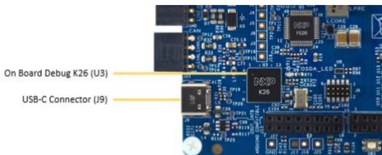
Figure 10. S32K312MINI-EVB - On board S32K3 Debugger
