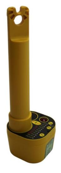
The wideband unit is designed to reliably detect voltages in the frequency range from 25Hz to 100Hz. It automatically compensates to provide stable and constant sensitivity for all frequencies in this range.
