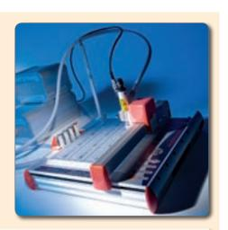
The MVPS-G3 series plotter can be simply and easily converted into a quality engraving machine complete with vacuum suction unit. Conversion is very straightforward: The spindle unit is affixed on the plotter in place of the pen unit and connected to the vacuum cleaner and a control unit for the spindle.
