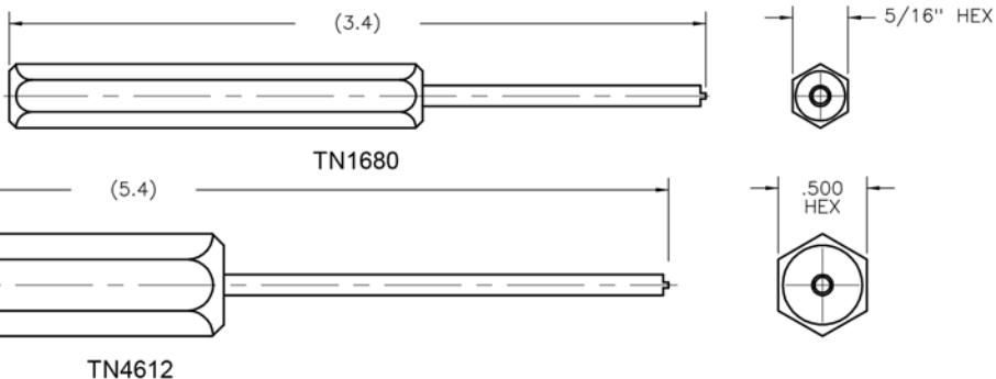
USING EITHER OF THE SPANNER WRENCHES SHOWN ABOVE, GUIDE SETS MAY BE REMOVED AND REPOSITIONED IN ANY OF THE 64 POLARIZING POSITIONS. REFER TO PAGE WA-18 FOR POLARIZATION CHART.
