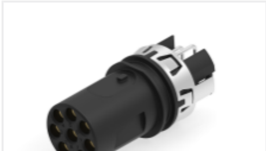
TE Part #225301-E M12 FEMALE, A CODE,RA, 8P THR REAR MOUNT
