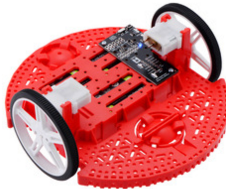
Power Distribution Board for Romi Chassis.
