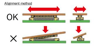
2) When fully aligned the connectors are parallel to each other with restricted longitudinal and lateral movement. Mate them parallel to each other.
