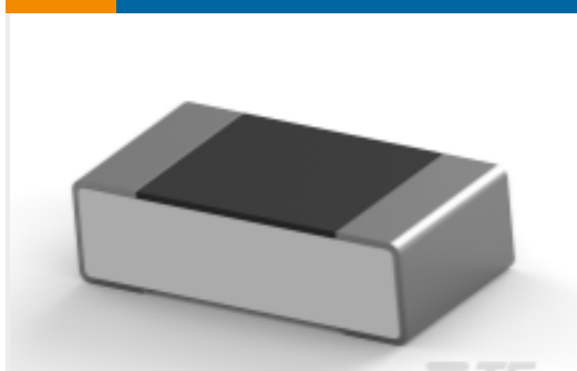
TE Part #3-2176370-4 RQ 0603 953R 0.1% 10PPM 5K RL
