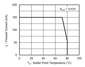
Fig. 1 - Maximum Forward Current vs. Solder Point Temperature
