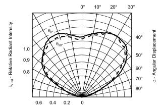
Fig. 5 - Relative Radiant Intensity vs. Angular Displacement
