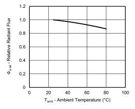
Fig. 6 - Relative Radiant Flux vs. Ambient Temperature
