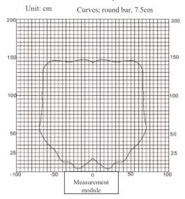
Note: The inner area of the arc or ultrasonic waves can be sensed to  $\varnothing 7.5 \mathrm{cm}$  round bar area
